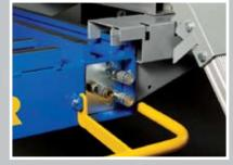
**Easy to handle;** multifunctional power unit and central satellite locations for hydraulics and air.
