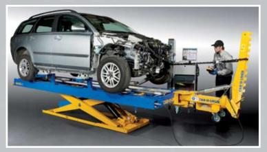
**Quality assured repairs** with accurate measuring in real time during the entire process by Car-O-Tronic.
