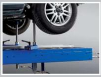
**Effective holding and clamping** and no need for extra fixtures when using EVO holding and anchoring system.
