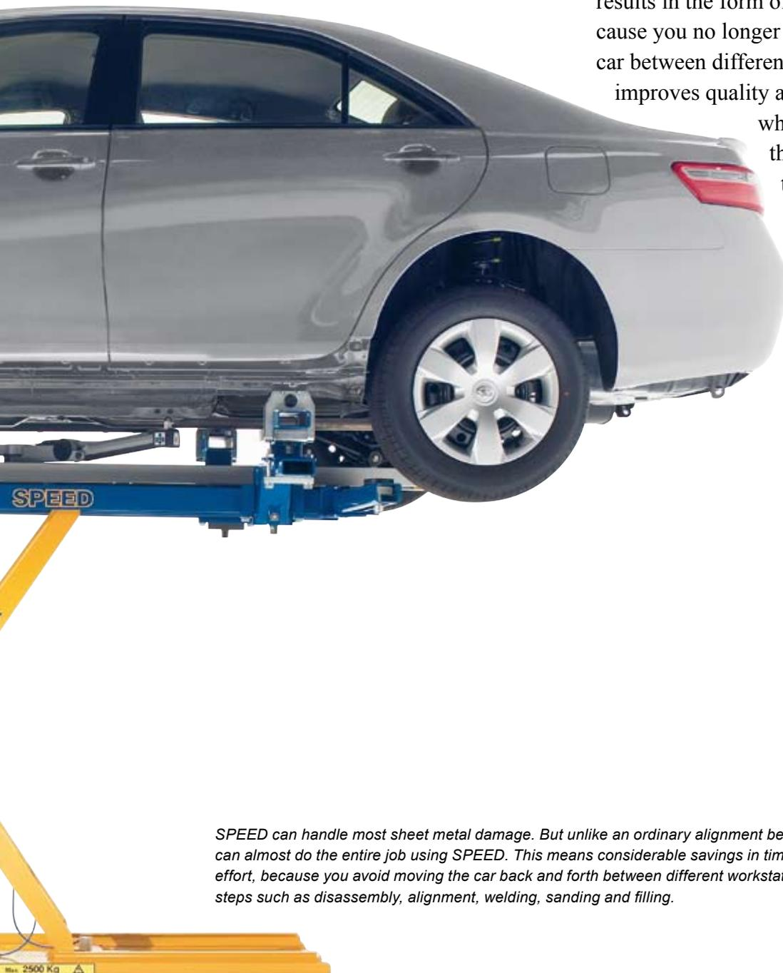
*SPEED can handle most sheet metal damage. But unlike an ordinary alignment bench, you can almost do the entire job using SPEED. This means considerable savings in time and effort, because you avoid moving the car back and forth between different workstations for steps such as disassembly, alignment, welding, sanding and filling.*
