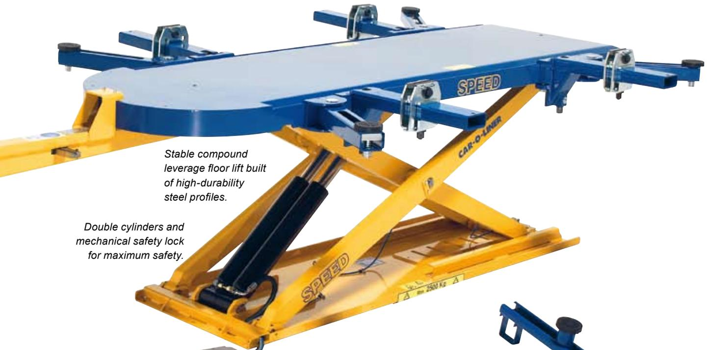
*Stable compound leverage floor lift built of high-durability steel profiles.*
